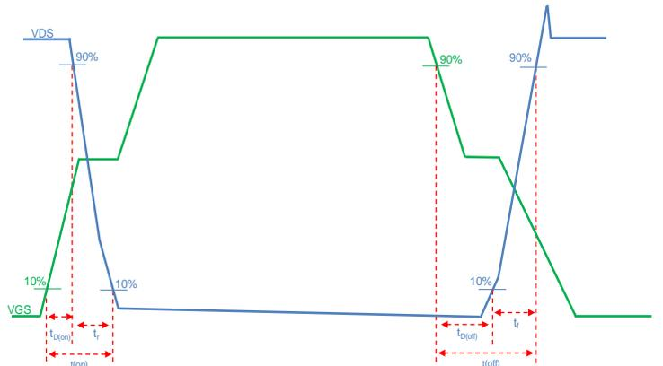
Figure C. Resistive Switching Test Circuit & Waveform
