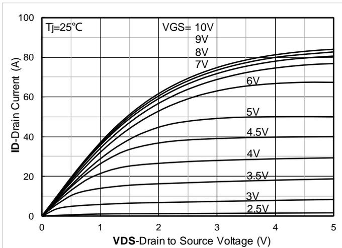
Figure 1. Output Characteristics
