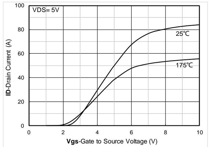
Figure 2. Transfer Characteristics
