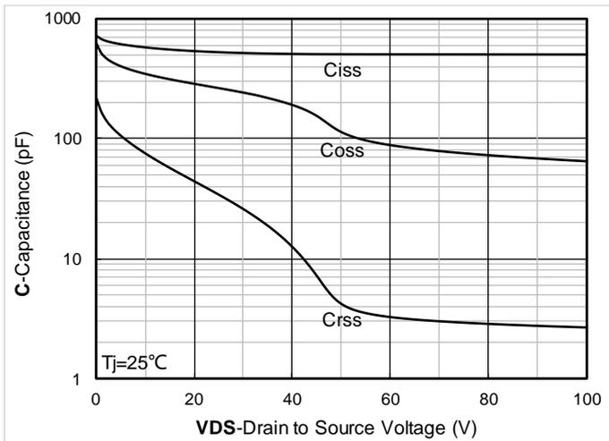
Figure 3. Capacitance Characteristics
