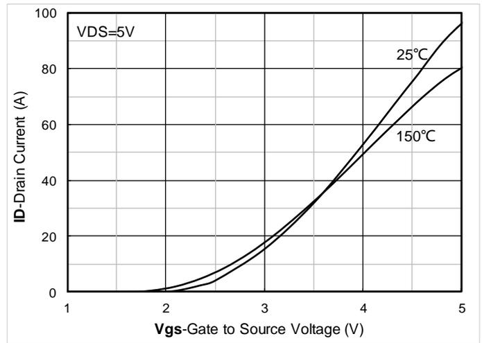
Figure 2. Transfer Characteristics
