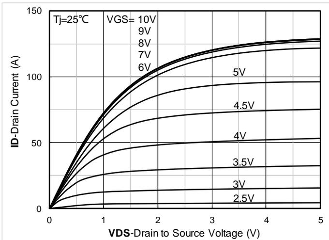
Figure 1. Output Characteristics
