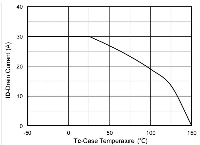
Figure 11. Current dissipation
