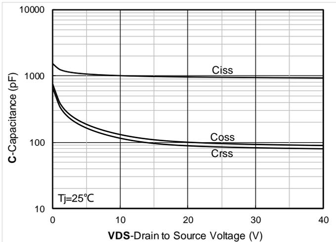
Figure 3. Capacitance Characteristics
